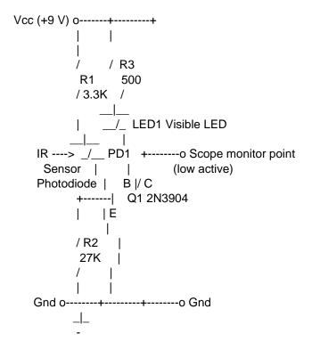
IR Detector Circuit Using IR Receiver Module
